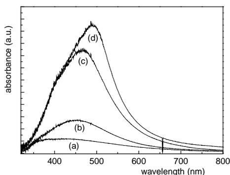
Fig. 2 : absorption spectrum of the ion-exchanged glass after UV exposure ( $40 \text{ kW/cm}^2$ ) and simultaneous heating : (a) room temperature, (b)  $260^\circ\text{C}$ , (c)  $350^\circ\text{C}$  and (d)  $450^\circ\text{C}$
