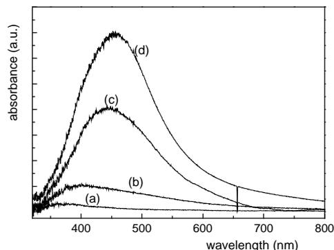
Fig. 1 : absorption spectrum of the ion-exchanged glass after UV exposure (25 kW/cm<sup>2</sup>) and simultaneous heating : (a) room temperature, (b) 260°C, (c) 350°C and (d) 450°C
