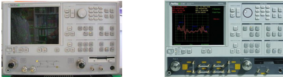
Fig. 3: real and remote interface of a device (network analyzer)
