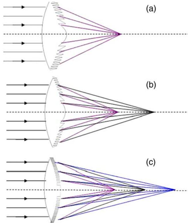
Fig. 1. (Color online) Three diffractive lenses used for Zemax simulations: (a) monofocal lens ( $P = +23\text{D}$ ), (b) bifocal lens ( $P = +20\text{D}/ +23\text{D}$ ), and (c) trifocal lens ( $P = +17\text{D}/ +20\text{D}/ +23\text{D}$ ).
