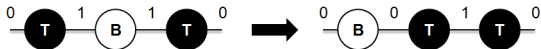
Fig. 4. Propagation of tokens and bubbles in STRs (tokens move to the right, bubbles to the left)
