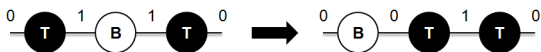
Fig. 4. Propagation of tokens and bubbles in STRs (tokens move to the right, bubbles to the left)
