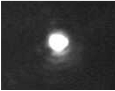
FIG. 3. Output light intensity of the hybrid structure (@1550 nm).
