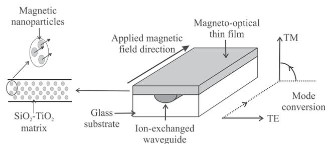
FIG. 1. Schematic of the integrated magneto-optical mode converter.
