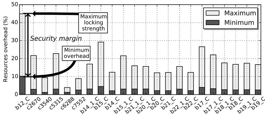
Fig. 16 Trade-off between locking strength and resources overhead
