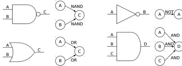
**Fig. 6** Conversion from logic gates to graph elements
