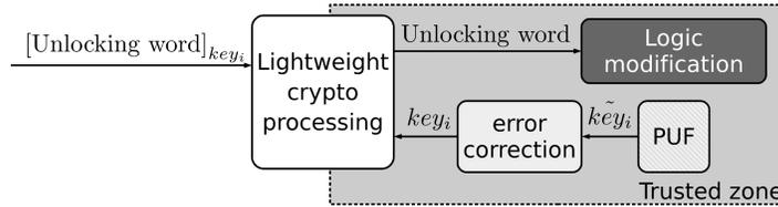
**Fig. 18** Architecture of the proposed design protection module
