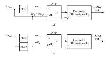
Fig. 1. PLL-based TRNGs using one (a) or two (b) PLLs
