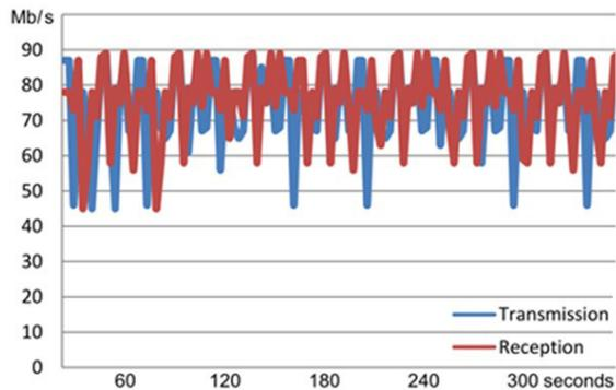
Fig. 11. TX and RX variation, frequency band 13 - 33 MHz.
