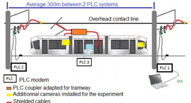
Fig. 1. Experimental installation of the tramway PLC link.
