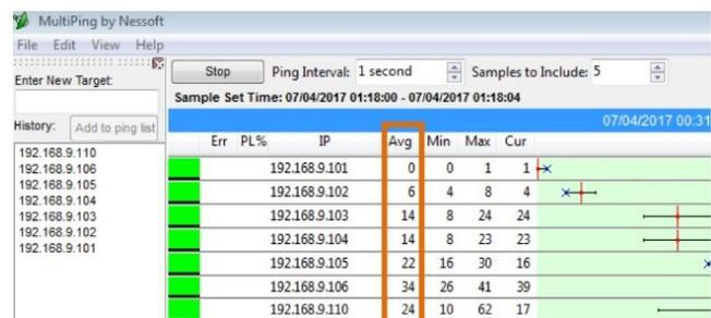
Fig. 12. RTT measured from the remote station.
