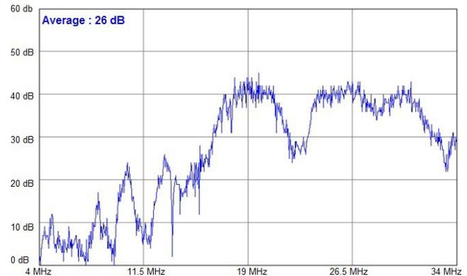
Fig. 4. SNR from the embedded PLC modem, freq band 4-34 MHz.
