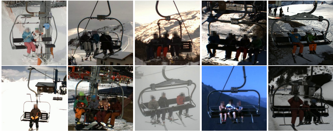
Figure 3: Example images from our chairlift dataset. The two left images are “open” class while the others are “close” class.
