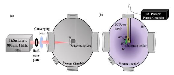
**Figure 1.** Experimental setup with the femtosecond laser beam focused into the vacuum chamber equipped with a plasma generator. (a) Irradiation of the W target inside a vacuum chamber. (b) Sputtering of the target surface prior to laser irradiation, in which the inert argon ion plasma created by polarizing the substrate holder using a continuous power supply provided by the pinnacle plus and the accelerated argon ions spray off the adsorbed oxide layer.
