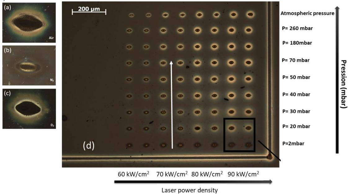
Figure 1 : pictures of laser spots written at 244 nm ( $\tau = 1 \text{ s}$ ): (a) Air ( $P_{\text{atm}}$ ), (b)  $\text{N}_2$  ( $P_{\text{atm}}$ ), (c)  $\text{O}_2$  ( $P_{\text{atm}}$ ). (d) increasing air pressures and laser power densities.
