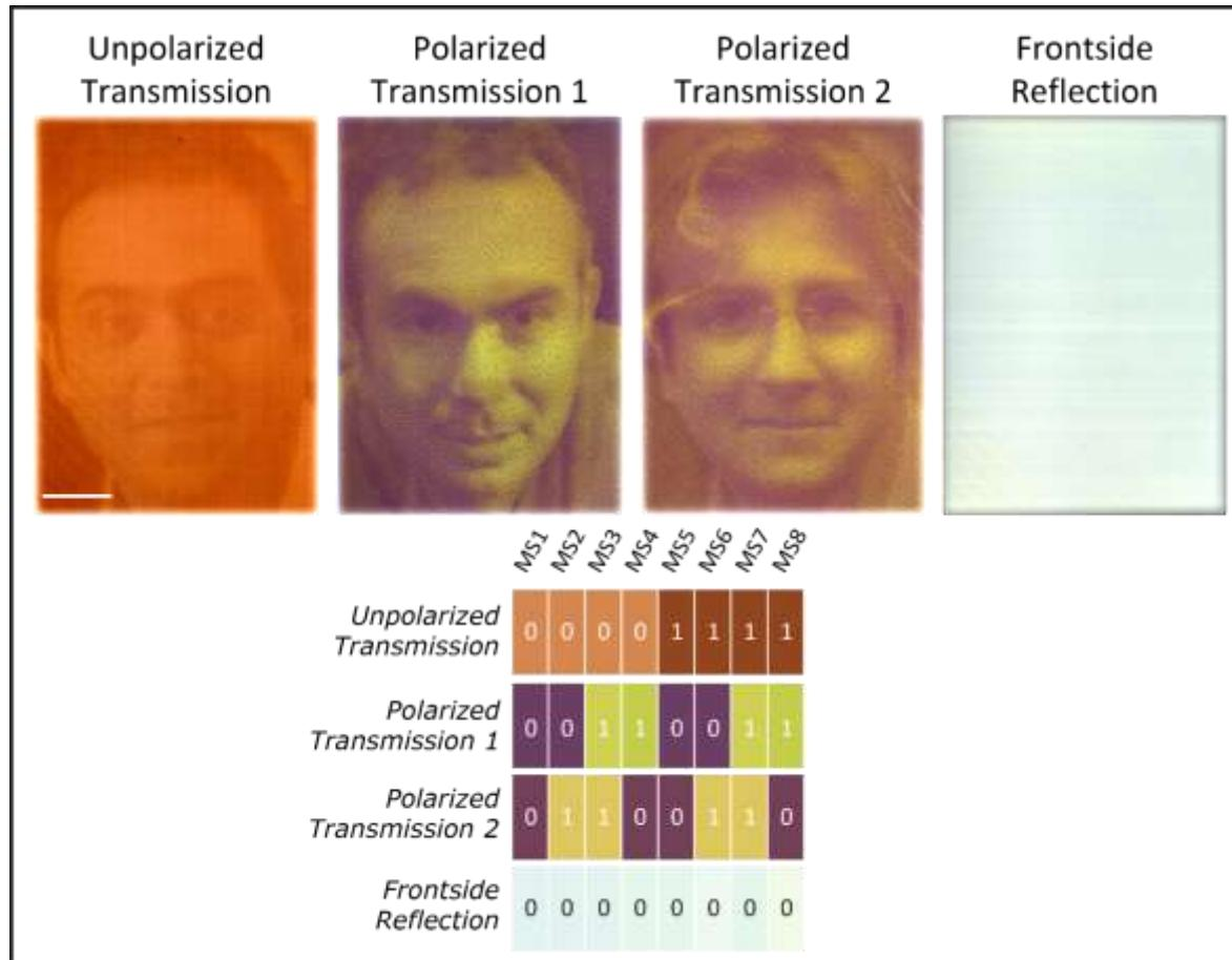
**Figure 7.** Four-image multiplexing with polarized white light. Three images and a blank image are multiplexed to be revealed in “unpolarized transmission”, “polarized transmission 1”, “polarized transmission 1” and “frontside reflection”. The pictures are the photographs of the sample taken with our setup in the corresponding modes. The colors of the eight metasurfaces are displayed in the logical color tree. The length of the scale bar is 2.5 mm.
