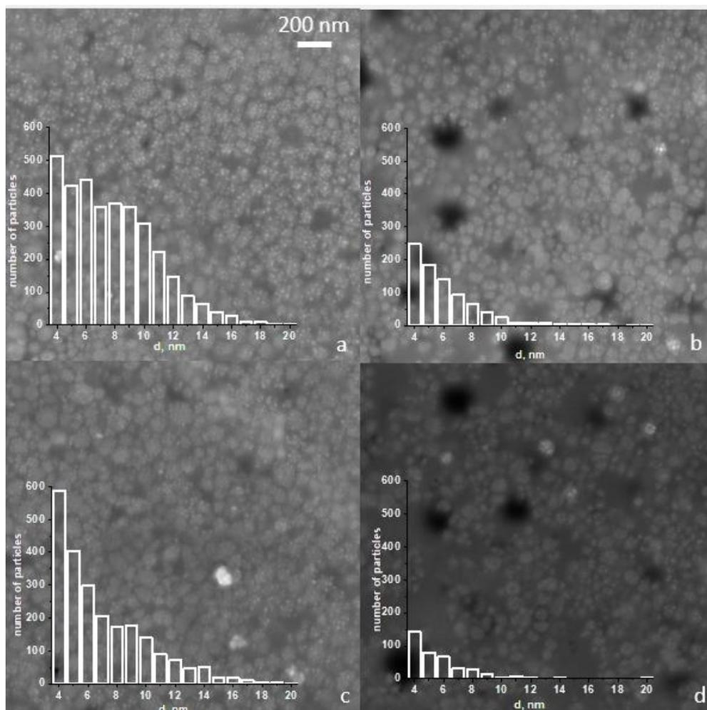
**Fig. 8.** SEM images of tracks. a)  $V_{sc} = 100 \mu\text{m/s}$ ,  $I_0 = 1.07 \text{ MW/cm}^2$ ; b)  $100 \mu\text{m/s}$ ,  $0.89 \text{ MW/cm}^2$ ; c)  $50 \mu\text{m/s}$ ,  $1.07 \text{ MW/cm}^2$ ; d)  $50 \mu\text{m/s}$ ,  $0.89 \text{ MW/cm}^2$ .
