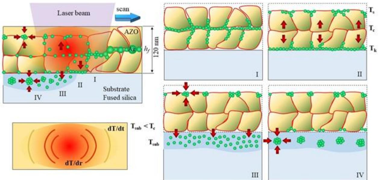
**Fig. 11.** The scheme of AZO:Ag film photothermal modification with the following stages: I. Decomposition of Ag NPs into monomers; II. mass transfer of Ag monomers from the center of the film to the surface and to the film-substrate interface; III. the outflow of Ag monomers from the film to the substrate during its softening, as well as the growth of Ag nanoclusters on the film surface; IV. agglomeration of Ag monomers and growth of NPs in the substrate.
