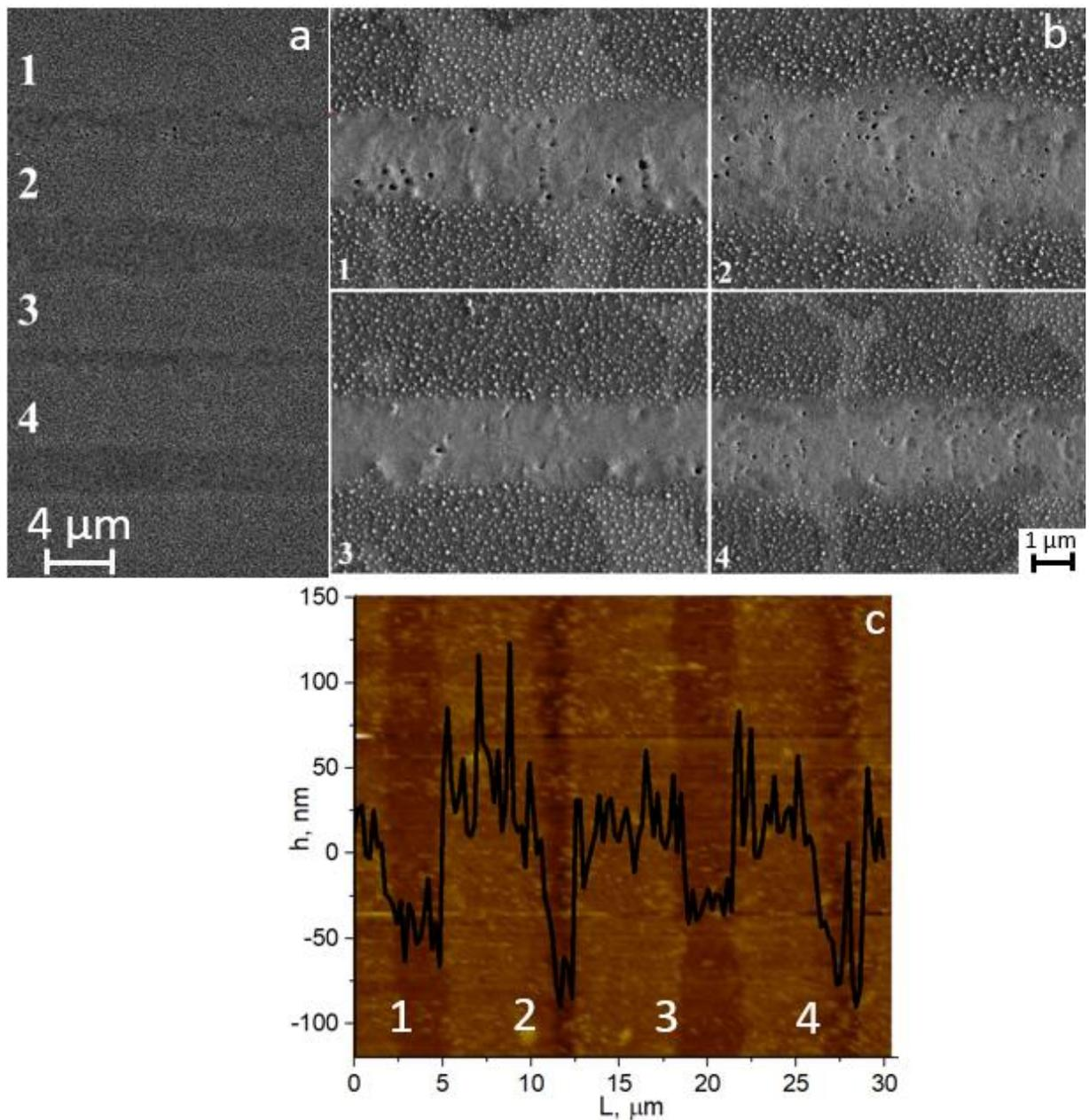
**Fig. 6.** (a) SEM images 1 –  $V_{sc} = 50 \mu\text{m/s}$ ,  $I_0 = 0.89 \text{ MW/cm}^2$ ; 2 –  $50 \mu\text{m/s}$ ,  $1.07 \text{ MW/cm}^2$ ; 3 –  $100 \mu\text{m/s}$ ,  $0.89 \text{ MW/cm}^2$ ; 4 –  $100 \mu\text{m/s}$ ,  $1.07 \text{ MW/cm}^2$ . (b) SEM images with higher magnification. (c) 2D image (top view) of the relief obtained with the SPM. The y-axis (h, nm) corresponds to the relief depth.
