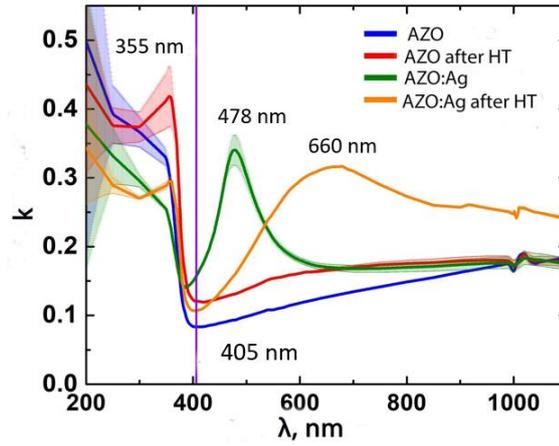
**Fig. 3.** Extinction of AZO and AZO: Ag films without HT and after HT in the furnace. Colored areas around the curves correspond to the error bars.
