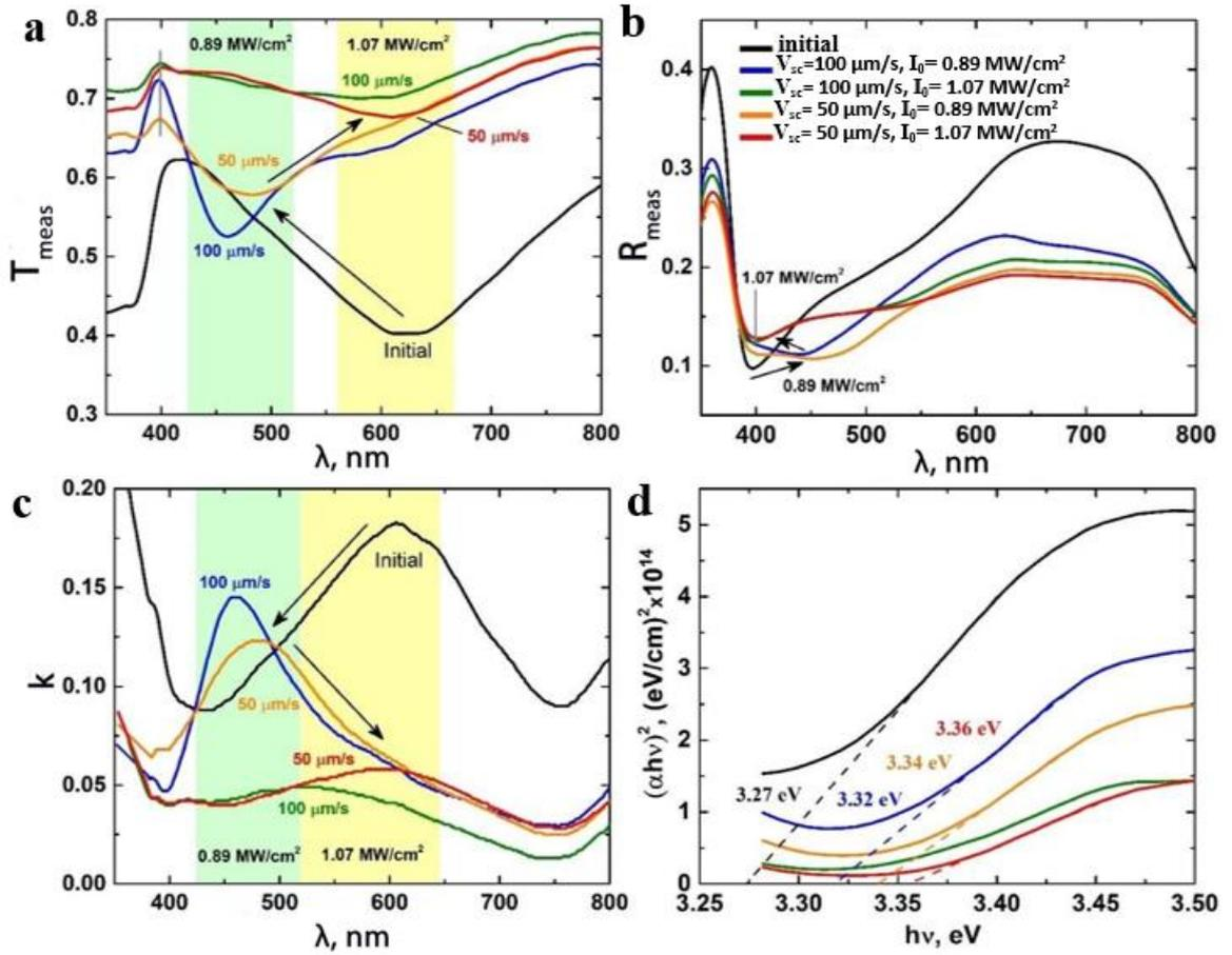
**Fig. 9.** Transmission (a), reflection (b), extinction (c), and curve  $(\alpha h\nu)^2$  (d) for the original film (black) and recorded tracks  $V_{sc}=100 \mu\text{m/s}$ ,  $I_0=0.89 \text{ MW/cm}^2$  (blue);  $V_{sc}=100 \mu\text{m/s}$ ,  $I_0=1.07 \text{ MW/cm}^2$  (green);  $V_{sc}=50 \mu\text{m/s}$ ,  $I_0=0.89 \text{ MW/cm}^2$  (orange);  $V_{sc}=50 \mu\text{m/s}$ ,  $I_0=1.07 \text{ MW/cm}^2$  (red).
