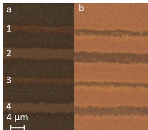
**Fig. 5.** Optical images of the recorded tracks. 1 –  $V_{sc} = 50 \mu\text{m/s}$ ,  $I_0 = 0.89 \text{ MW/cm}^2$ ; 2 –  $50 \mu\text{m/s}$ ,  $1.07 \text{ MW/cm}^2$ ; 3 –  $100 \mu\text{m/s}$ ,  $0.89 \text{ MW/cm}^2$ ; 4 –  $100 \mu\text{m/s}$ ,  $1.07 \text{ MW/cm}^2$ ; (a) Tl, (b) Rl.
