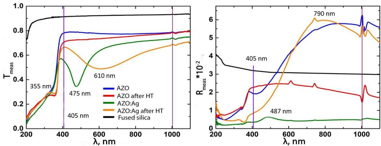
**Fig. 2.** Transmission (left) and reflection (right) of AZO films without HT (blue curve) and after HT in the furnace (red curve), as well as AZO:Ag without HT (green curve) and after HT in the furnace (orange curve).
